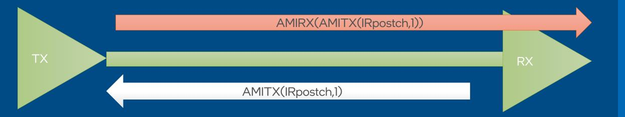
• TX AMI\_Init takes its unequalized "post-"channel. RX takes its potentially TX-equalized "pre-" channel indicated by the pink background.
